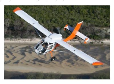
The engine placement allows the pilot and co-pilot to fly with 270° of visibility. The airplane has docile handling characteristics that provide for a safe, low-speed stall, responsive harmonized control, minimal pitch change with power and flap changes, and stability to reduce pilot workload, company officials said, noting it is easily configured for a variety of surveillance and sensor equipment.
