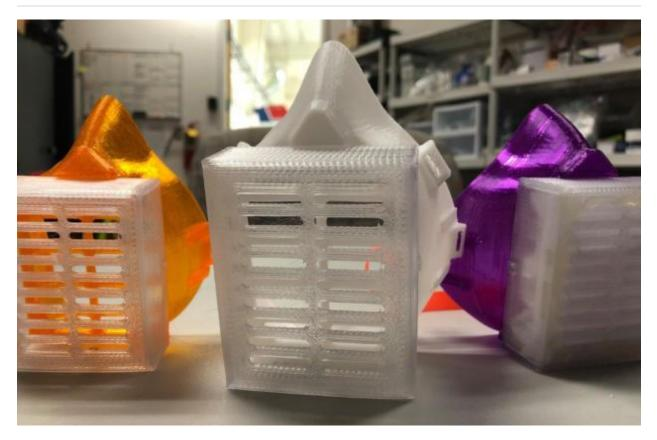
Masks 3D-printed at the University of New Mexico COSMIAC lab are made of thermoplastic polyurethane, or TPU, a durable but pliant material that adheres to the contours of the face. Two layers of filters go into the attached boxes. (Courtesy of Laura Kief Shaffer)
